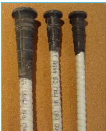
GFRP bars with anchored heads.
