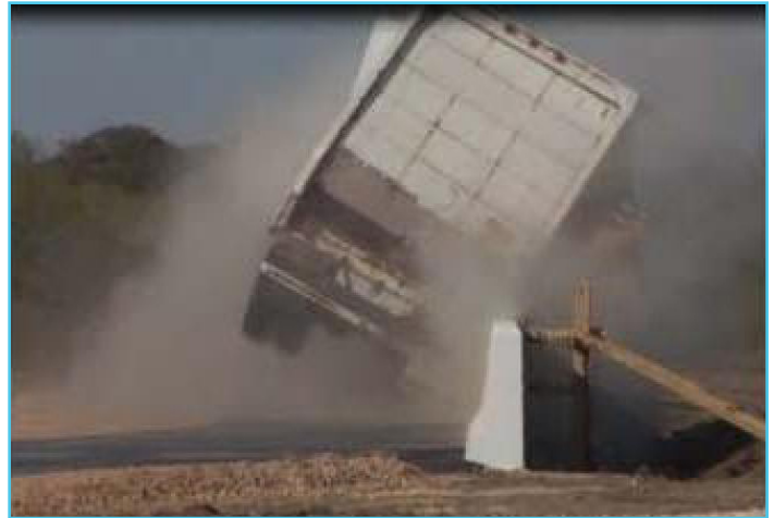
PL-3 barrier tests require impact by a tractor trailer.
