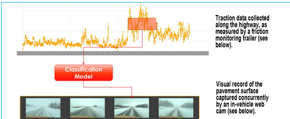
Figure 2a: Automated conversion of traction measurements to snow cover class.
